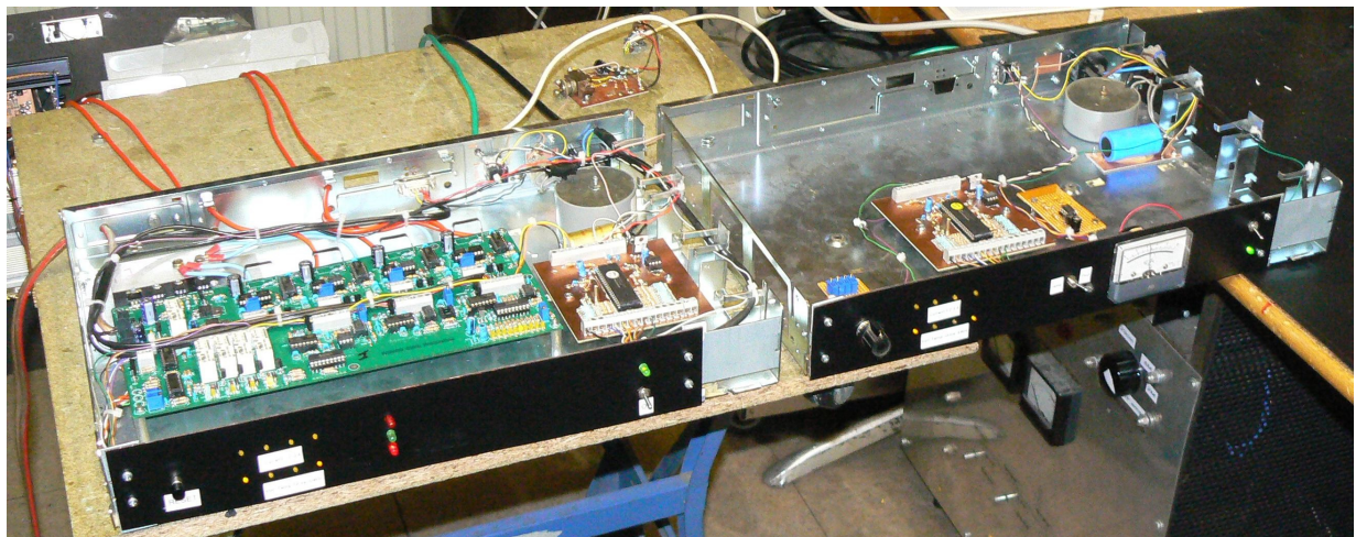
17: The indoor and remote unit side by side
