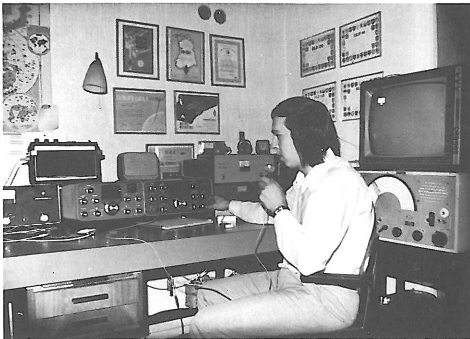
Fig. 13. Rheinhard Koch, DK1KO, at his operating position. Rheinhard's 144 MHz antenna array consists of four 16-element Yagis with a gain of about 22 dB. His final amplifier uses a pair of 4CX250B tubes.
