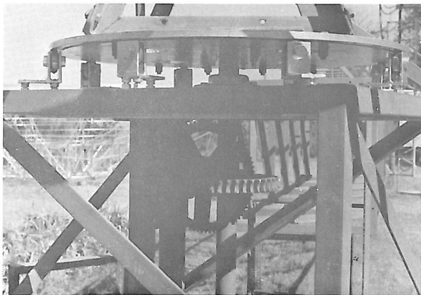
AX axis worm drive, rotary turntable and upturned ball races.
