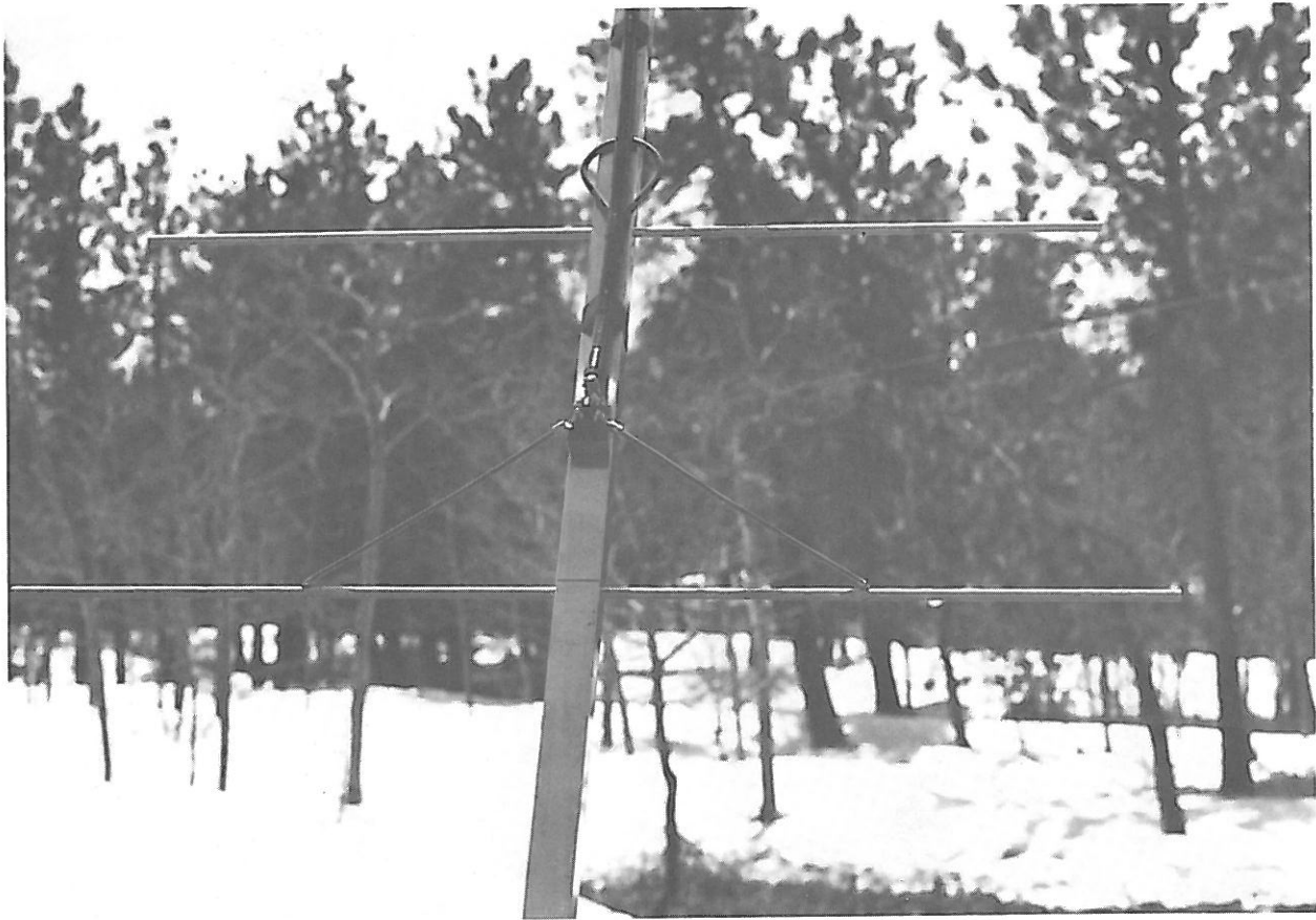
View of delta matched dipole element and balun.
