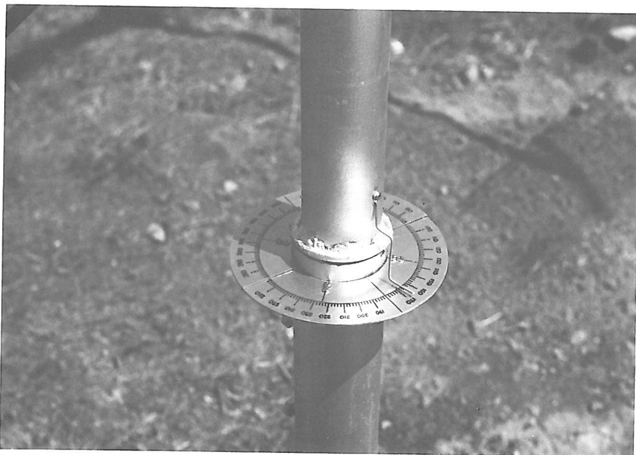
Main bearing, vertical support and azimuth calibration disc.
