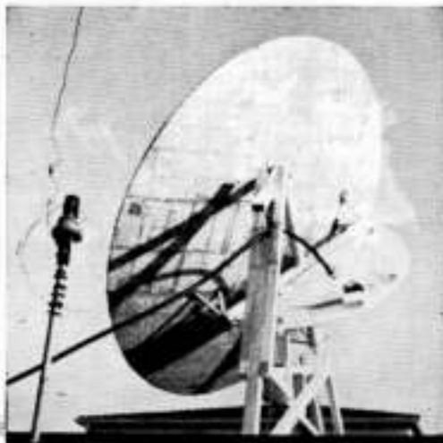
Mounted on the roof of his Los Angeles home, this is the homemade dish of WB6IOM. He used this dish to successfully work G3LTF and establish a new 1296-MHz. moonbounce record. The 16-foot diameter dish consumed 450 square feet of sheet aluminum and 70 pounds of epoxy to bond the aluminum sheets. (WB6IOM photo)
