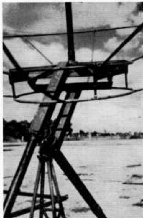
Shown is the hub assembly of the VK3ATN dish. The declination and hour angle drive motors are yet to be mounted as is a 16-inch diameter bearing.
