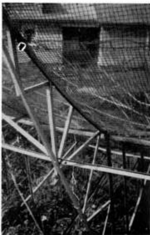
W3SDZ used hardware cloth for the covering on his 432-Mc. dish. Note the construction of the struts and supports.
